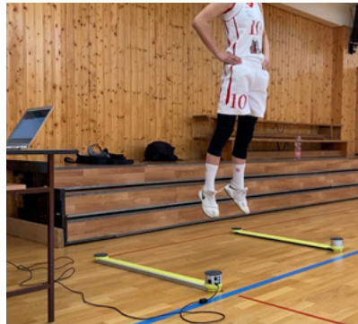
Picture 1 Vertical jump testing by OptoJump
