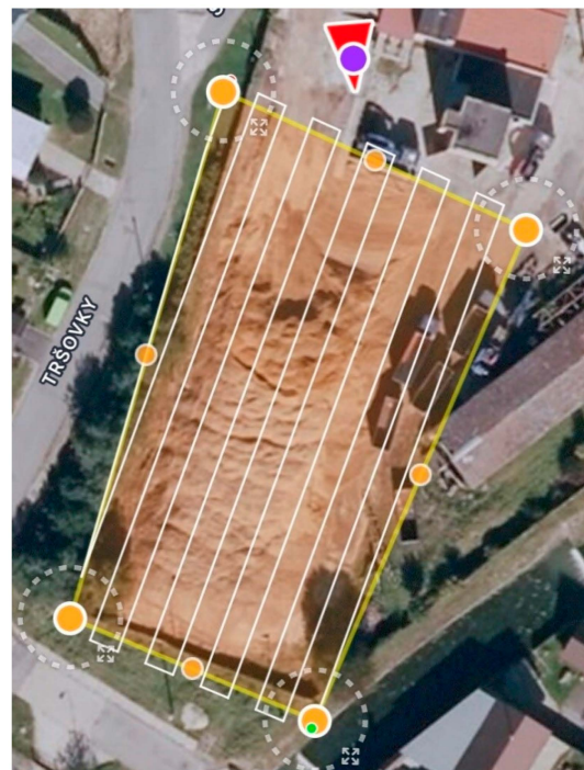
Figure 7. DJI Air 2S flight plan from Map Pilot Pro app.
