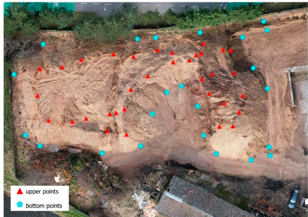
Figure 4. Location of GNSS Stonex S700A receiver-measured points.
