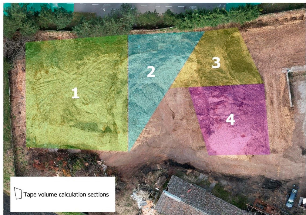
Figure 10. Dividing the pile into sections.
