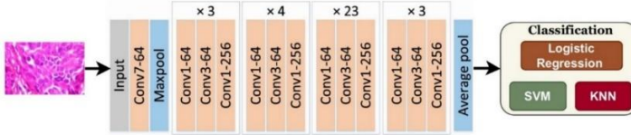
(c) ResNet101: Feature extraction with custom classification
