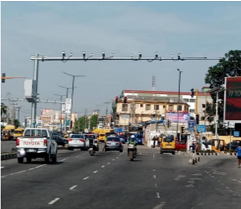
Figure 2 . Automatic Number Plate Recognition (ANPR) cameras in Lagos State (Olagunju, 2023)
