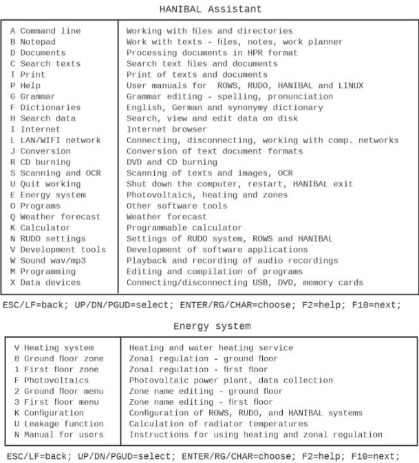
FIGURE 2. The top screen is the main screen with an overview of the main thematic modules offered by the RUDO system. The bottom screen is a sub-screen (accessible from the main screen by pressing the E key) with an overview of the main functions offered by the energy subsystem administration module. All text is translated from Slovak.
