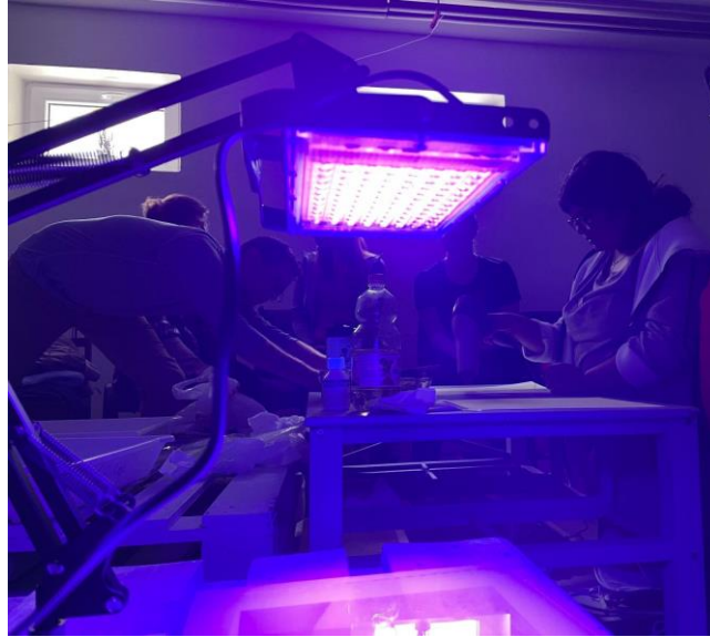
Figure 4. An ultraviolet lamp exposes the image during cloudy or rainy days when sufficient sunlight is unavailable.
