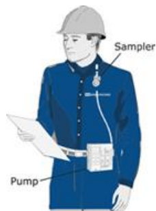
Obr. 18 Umiestnenie osobného prachomera (sampler) s pumpou (pump)( http://www.swtestingltd.co.uk/airsampling.html )
